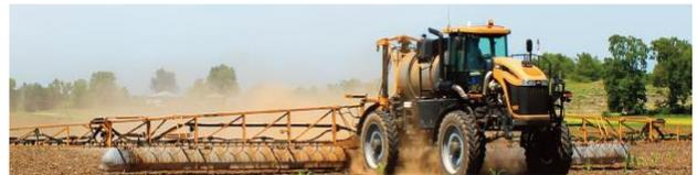
*"The concept is simple. If you spray inside an enclosed chamber there is less chance for wind to disrupt the spray pattern,"* explains Steve Claussen, president of Willmar Fabrication LLC – the manufacturer of Redball-Hooded™ Sprayers. *"Since the wind doesn't have access to the spray, more of the spray hits the targeted pest so growers get more value out of the spray he is paying for because he has less particle drift."*
