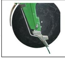
The Totally Tubular system shown in the picture to the right provides a much more efficient means of applying starter.
